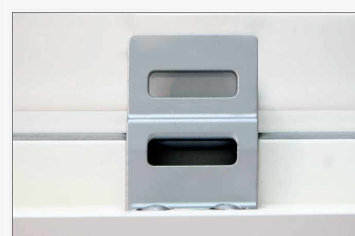
Ventilation position. The striking plate allows a 5mm night ventilation opening for all espagnolette handles.
